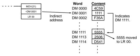
When using indirect addressing, the address of the desired word must be in BCD and it must specify a word within the DM area. In the above example, the content of \*DM 0000 would have to be in BCD between 0000 and 1999.
